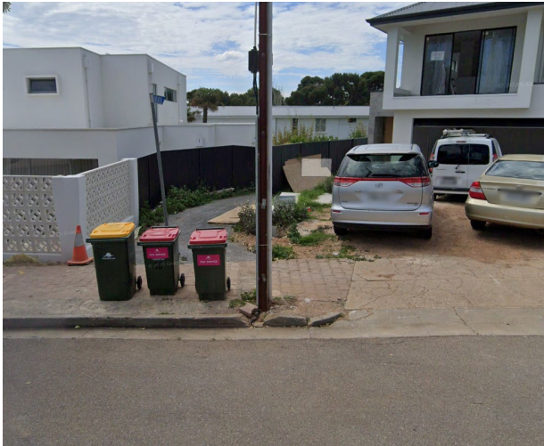
Image 2: Laneway view from Seaview Avenue Non-Trafficable due to barrier kerb, stobie pole, and street signage present at roadside
