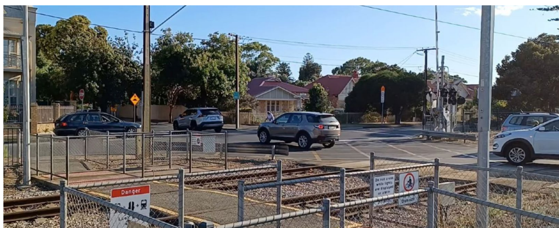
Cars travelling north – if first car has to give way at slow point the others will queue across the intersection
