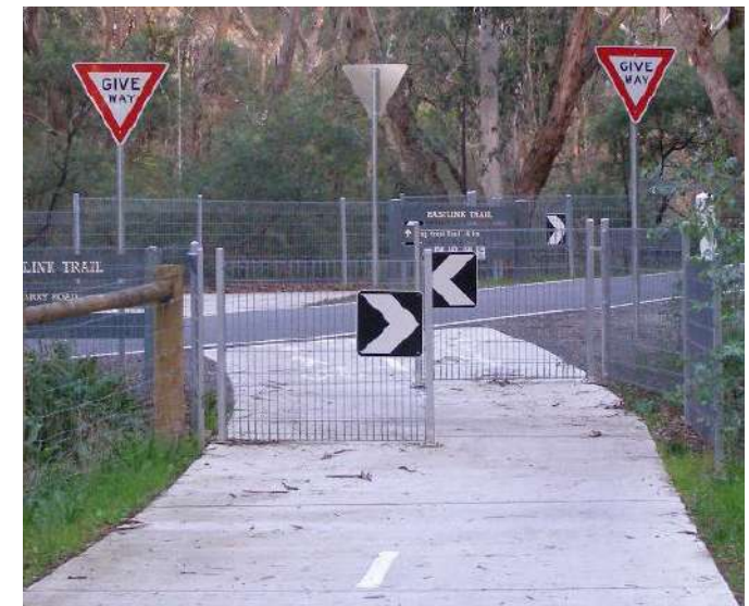
Staggered fence example
