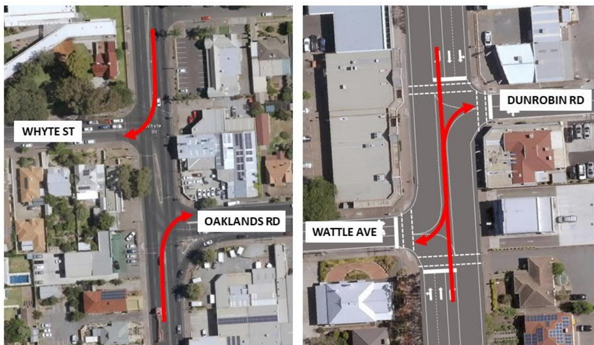
Figure 30 Comparison with Brighton Road, Oaklands Road and Whyte Street staggered intersection
