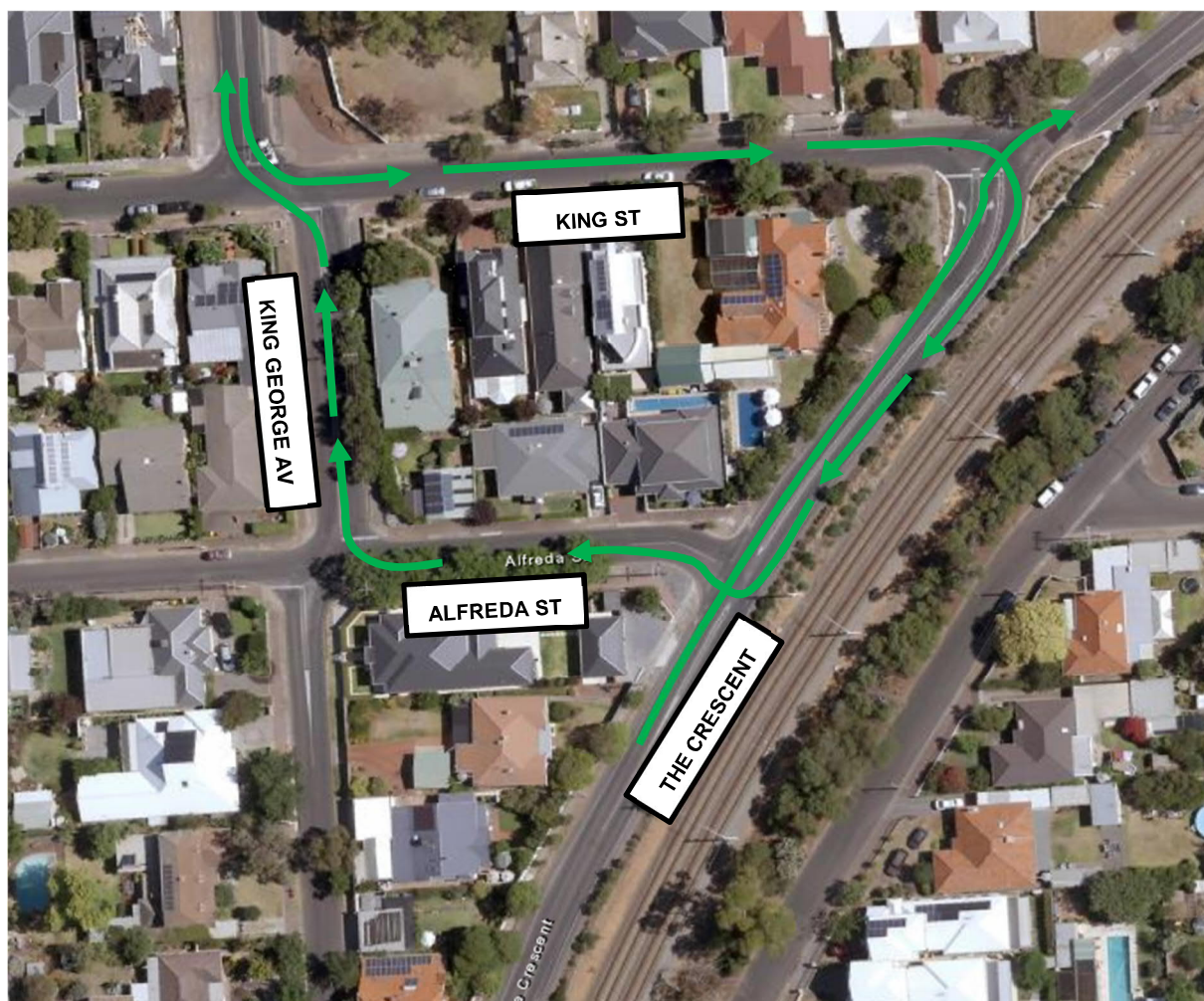
Figure 37 Proposed circuitous one-way arrangement
