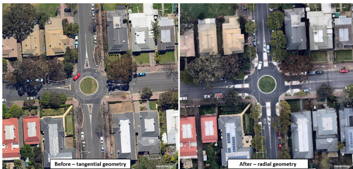
Figure 38 Example roundabout upgrade – intersection of Rugby St & Edmund Ave, Unley (Source: Nearmap)
