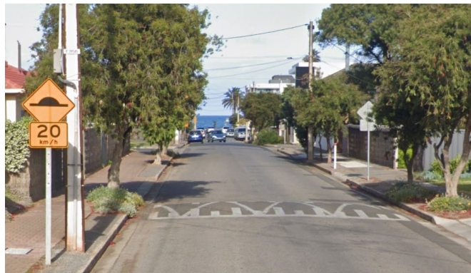
Example of road humps
